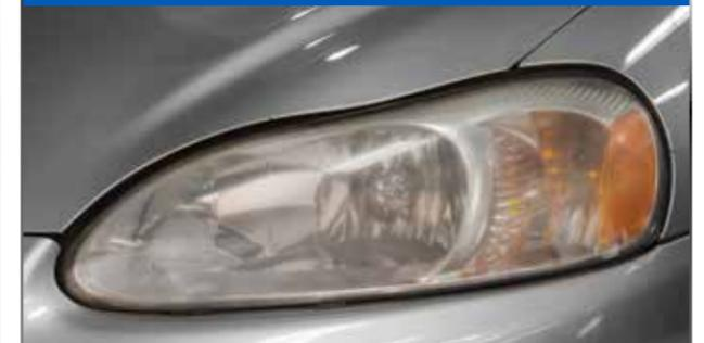
Scratch refinement can be accomplished by progressive sanding followed by a Lens Drier application to achieve a finish optimal for sealant.
