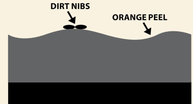
**REMOVING THE DEFECTS**
