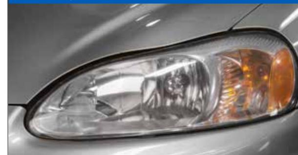
The wipe-on sealant provides a lasting protection to the polycarbonate lens.
