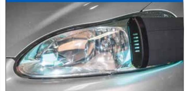
Use natural sunlight or the Presta UV Curing Light to cure the sealant on the restored lens. Headlight lenses properly restored with ReNuLite will last 1 year or more with the wipe-on application.
