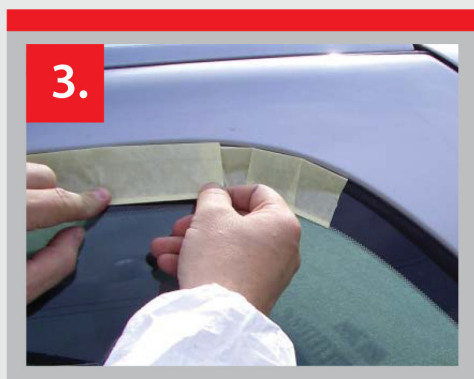
3. To mask along a straight section, tear off a section no longer than 20cm, slide in and leaver back the trim ensuring it overlaps the last piece.
